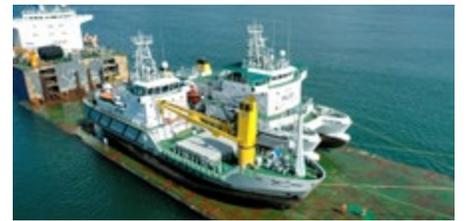
*Buoy Tender Vessel (BTV) & Pilot Station Vessel (PSV) -Loaded to the heavy lifter*
